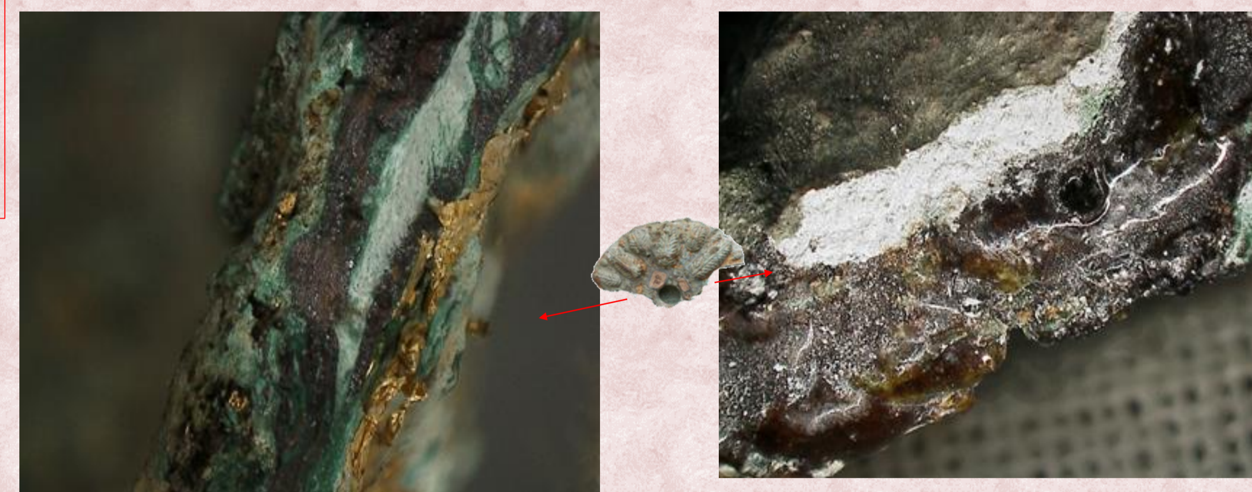
Figure 5. figure of Optical microscopy: detailed stratigraphy. Figure 6. of Optical microscopy: shellac and CaSO 4 .
