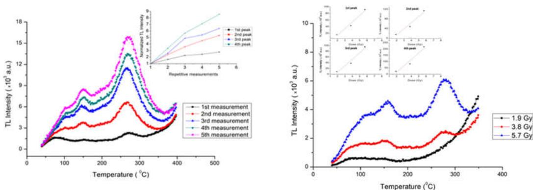
Fig1: a) Sensitivity test on the dihydrate calcium sulfate, b) Dose Response of the dihydrate calcium sulfate
