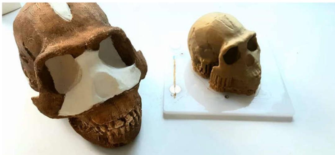
In order to 3D print the duplicate, an Einstart C printer was used. The model was scaled down to 65% of the original dimensions. The layer height of 0.1mm was selected in order to preserve most of the details.
